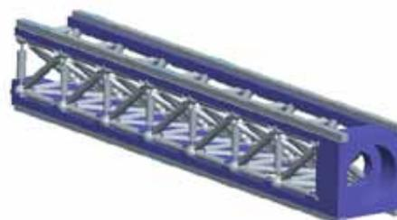
Figure 3. New reticular design of the ram made of carbon-fibre bars
