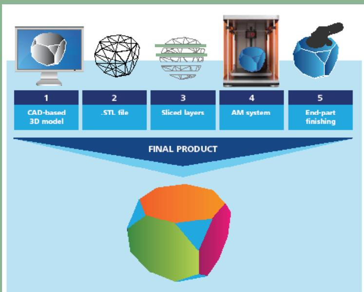
Figure 2 – The AM standard process
