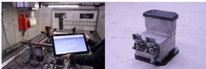
Testing in TYC FPPC 250/6 CNC machine tool and a detail of the active fixture unit
