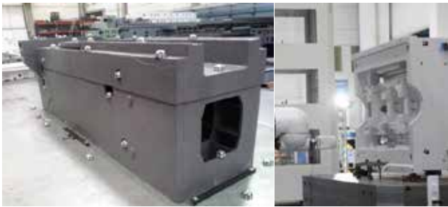
Part to be machined with photogrammetric markers (left, out-of-machine; right, on-machine)
