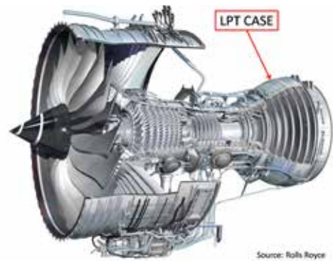
Workpiece under assessment and location in the turbine
