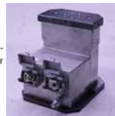
CAD models and realisation of active positioning units for workpiece automatic levelling and pre-deformation
