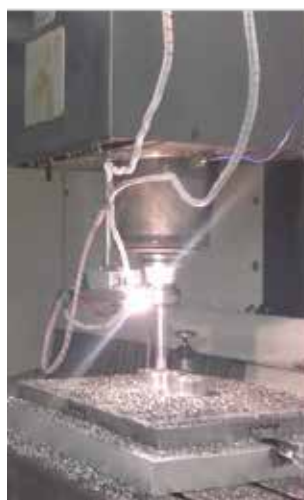
Chatter vibration mitigation and increased productivity results on industrial test-case
