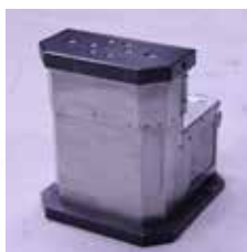
CAD models and realisation of active positioning units for workpiece automatic levelling and pre-deformation
