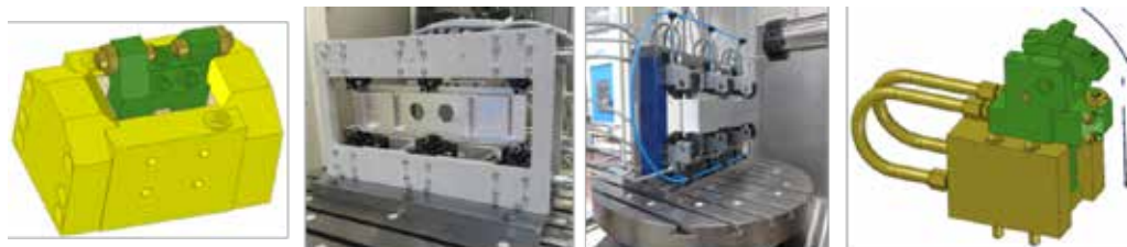
'PosiFlex' floating clamp (2x 6 mm; 7 kN at 250 bar)
