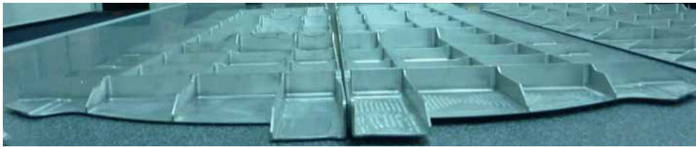
Parts manufactured with the same machining process. Notice the different distortion on both parts
