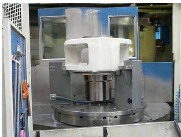
Implementation of the active fixture and the Mida WRS touch probe system into the lathe machine
