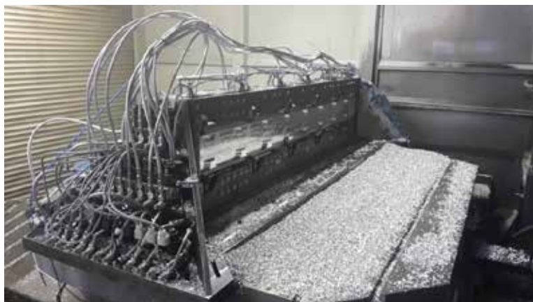
Final intelligent fixture prototype (CAD design and application in industrial environment)
