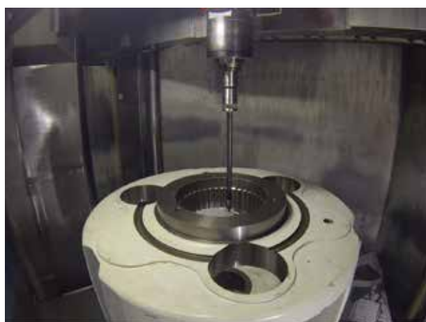
Implementation of the active fixture and the Mida WRS touch probe system into the lathe machine
