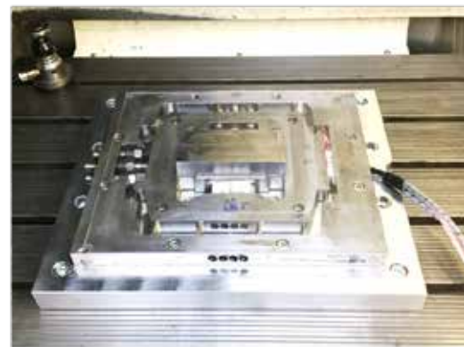
Manufacturing and assembly of the active fixture prototype equipped with sensors and actuators
