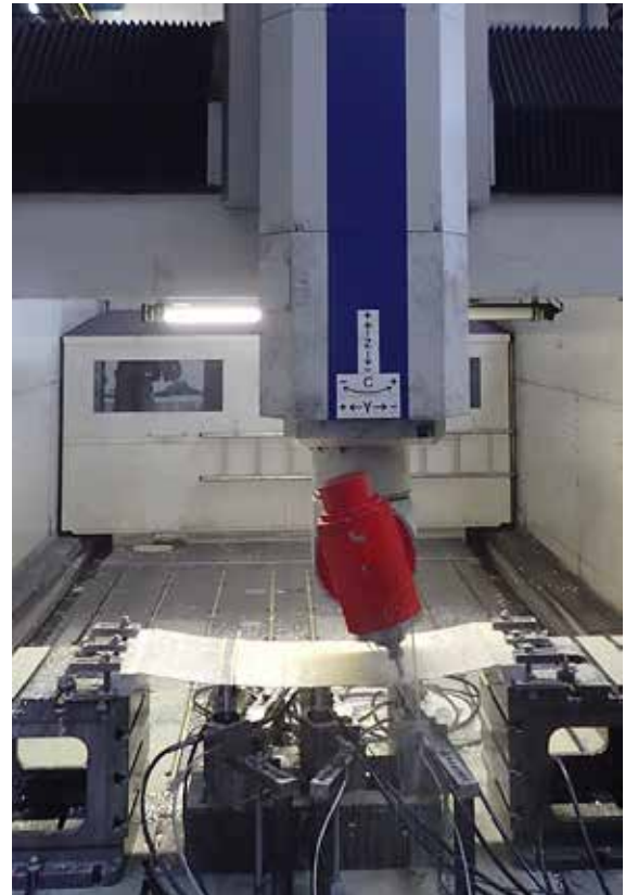
Demonstration thin-walled part machining under real conditions with adapted NC code
