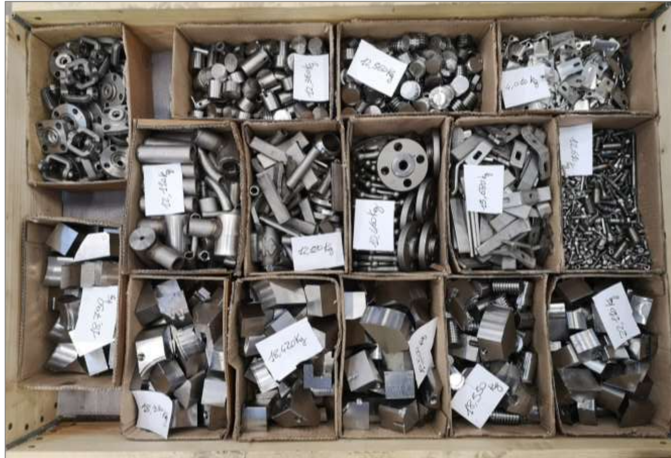
Metal scrap ready to be atomized
