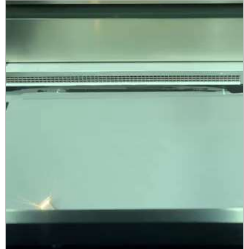
Printing of specimens and parts in LB-PBF systems (Concept Laser by GE and M290 by EOS)
