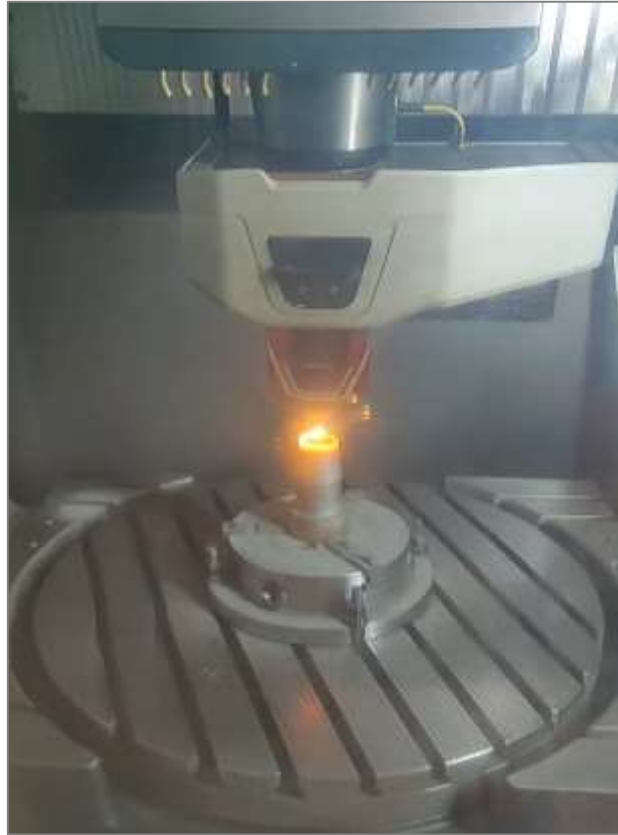
Printing of specimens in the L-DED machine (LASERTEC Hybrid by DMG Mori)
