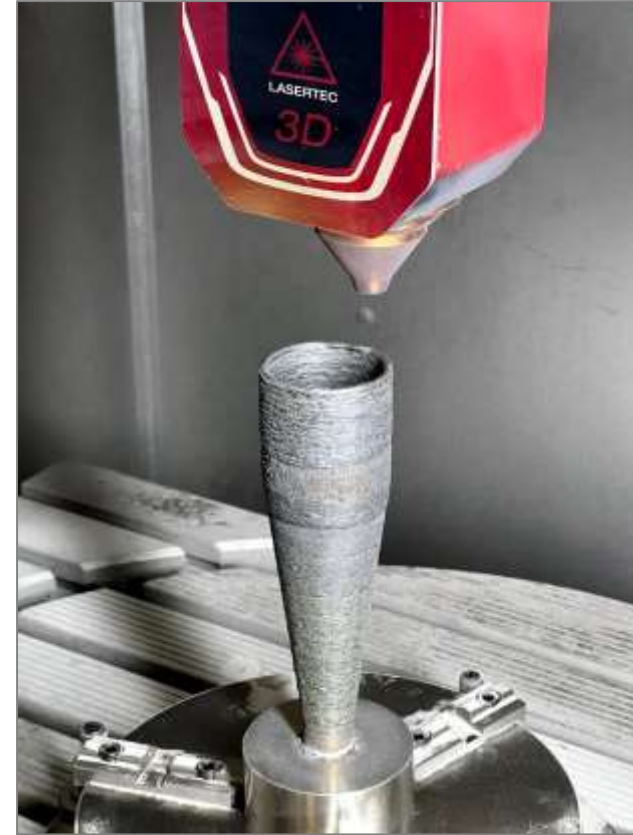
Printing of specimens in the L-DED machine (LASERTEC Hybrid by DMG Mori)
