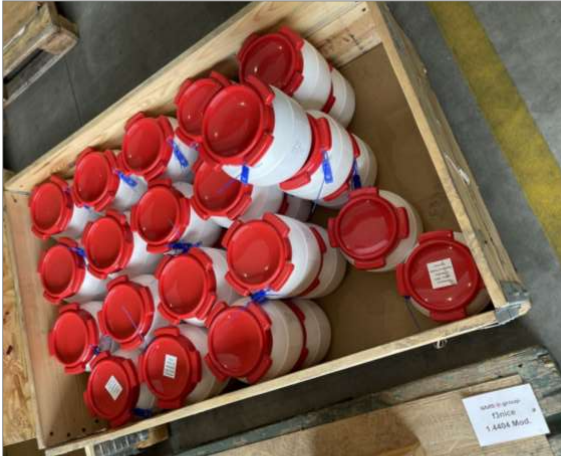
316L SS powder after atomization & sieving
