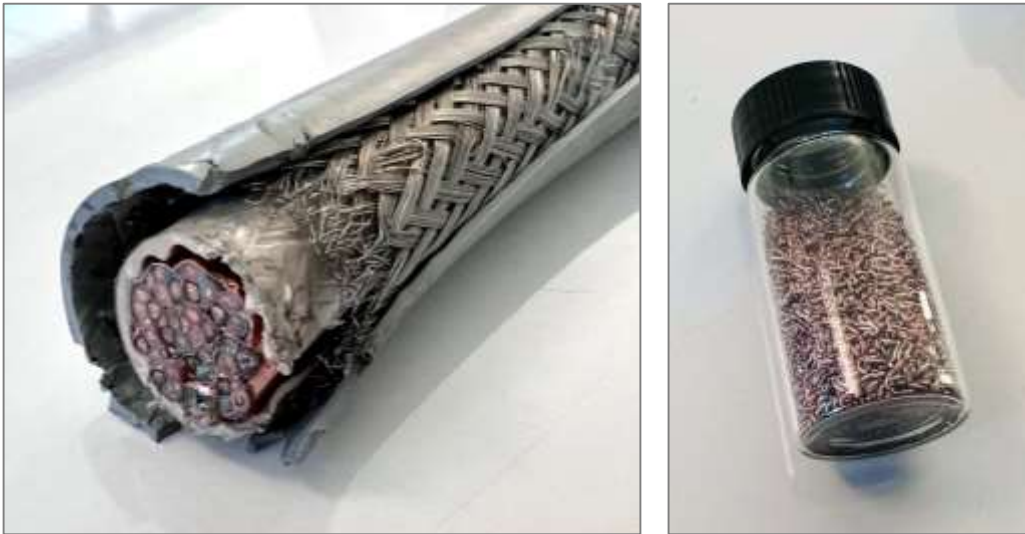
Copper retrieved from Sub Sea electrical cables
